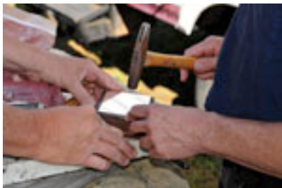
Tacking Plate to Board for Polishing Formulary Staff
